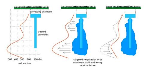
Diagrammatic illustration of how the intervention trench will work. To the left of the trench – the area closest to the trees – root induced negative porewater pressures will draw moisture from the treated zone beneath the conservatory. The trench is designed to satisfy the water demand and ensure the ground beneath the conservatory remains stable.
