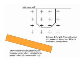
We are currently rehydrating the ground beneath a conservatory damaged by root induced clay shrinkage. The trees that have caused the damage are to be retained. The soil has a PI of 34%.
